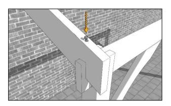
Butt the other rafter against the outer face of the post before securing in place with a 120mm coach screw driven down into the runner.
