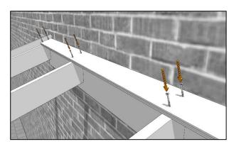
Take the short tongue and groove ridge (with no tongue), groove side facing down the roof and position it at the top of the rafters before fixing into place with:
