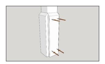
To attach cladding panels simply align as shown at the base of the post before screwing into place using 4 x 60mm woodscrews through the pre-drilled holes per panel. Repeat for each face of the post.
