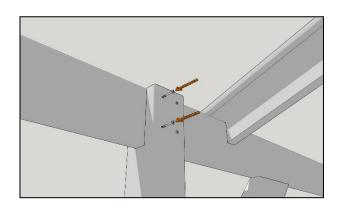
... before securing it into place with 2 x 60mm screws through the post into the runner.
