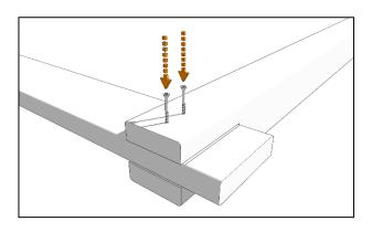
Place one of the posts on a flat surface as shown and then insert one of the runners into the post slot, using the markings on the runner as a guide. Fix into place with 2 x 60mm woodscrews.
