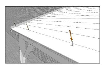
Add the final short tongue and groove panel before fixing into place with a 40mm screw into each rafter spaced 20mm from the top edge of the panel.
