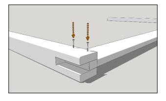
Slot another post over the other end of the runner, aligning with the single mark on the runner top edge and fix into place with  $2 \times 60 \text{mm}$  woodscrews.
