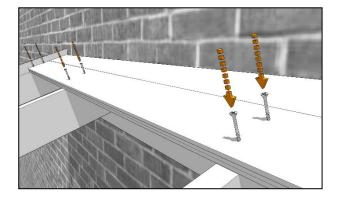
...before fixing into place with 2 x 40mm screws into each rafter, spaced 20mm from the upper and lower edges.
