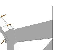
Place an end brace against the inner face of the outer runner so that the lower face is butted against the inner face of the post and the top edge is approximately 10mm from the top edge of the rafter. Fix in place with 1 x 70mm coach screws into the rafter and 2 x 50mm coach screws into the post as shown. Repeat for the other end of the structure.
