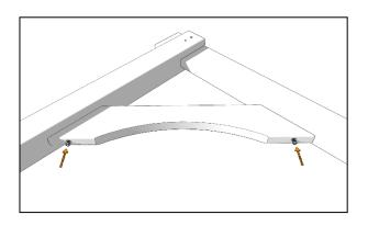
Align a brace with the underside of either end of the runner and centrally across the inside face of the post as shown. The mating faces should be flat against each other before fixing the brace into place with a 70mm coach screw at each end. Repeat and attach the remaining brace to the other end of the runner to form a "goal post" structure.
