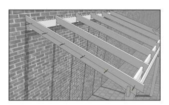
...and fix into place with 40mm screws.
