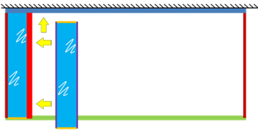
Inserting Next Glazing Panel Assembly
